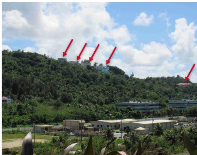
Figure 2: Homes located on a ridgeline, like these in Saipan (indicated by red arrows), typically experience higher wind speeds than homes on lower, flat terrain. See map in Figure 1 also.
