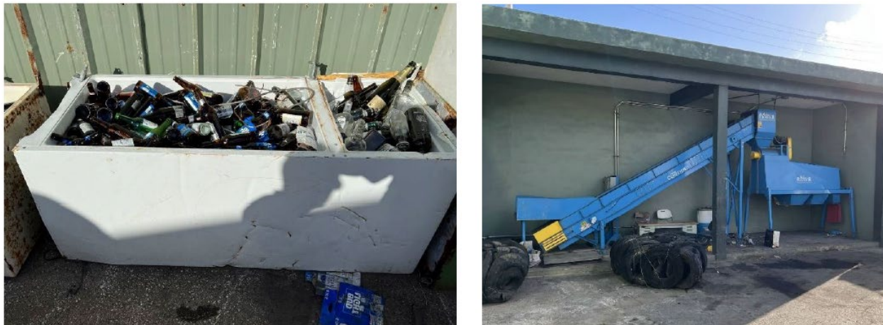
Figure 11 Glass Crusher and Collection Bin
