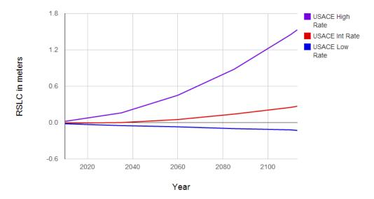
The original NRC curves result in global SLC values, by the year 2100, of 0.5 meters, 1.0 meters, and 1.5 meters. The USACE SLC calculator modified these curves to include the historic global MSL change rate of 1.7 mm/year and the start date of 1992 (which is the midpoint of the current National Tidal Datum Epoch of 1983-2001), instead of 1986 (the start date used by the NRC). This resulted in updated values for the calculator coefficients.
