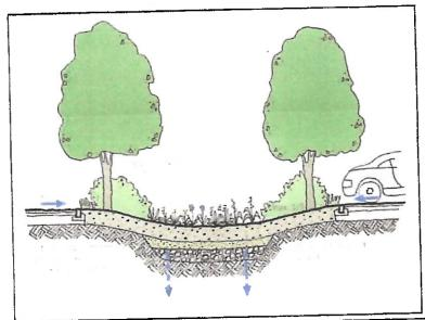
Bio retention areas (figure 1) are vegetated areas with specially designed engineering soils and sand layers, which filter out pollutants from surface water runoff normally associated with highways. Bio retention features have an aesthetic and biodiversity value as they can be planted to enhance local character and are attractive landscape features.
