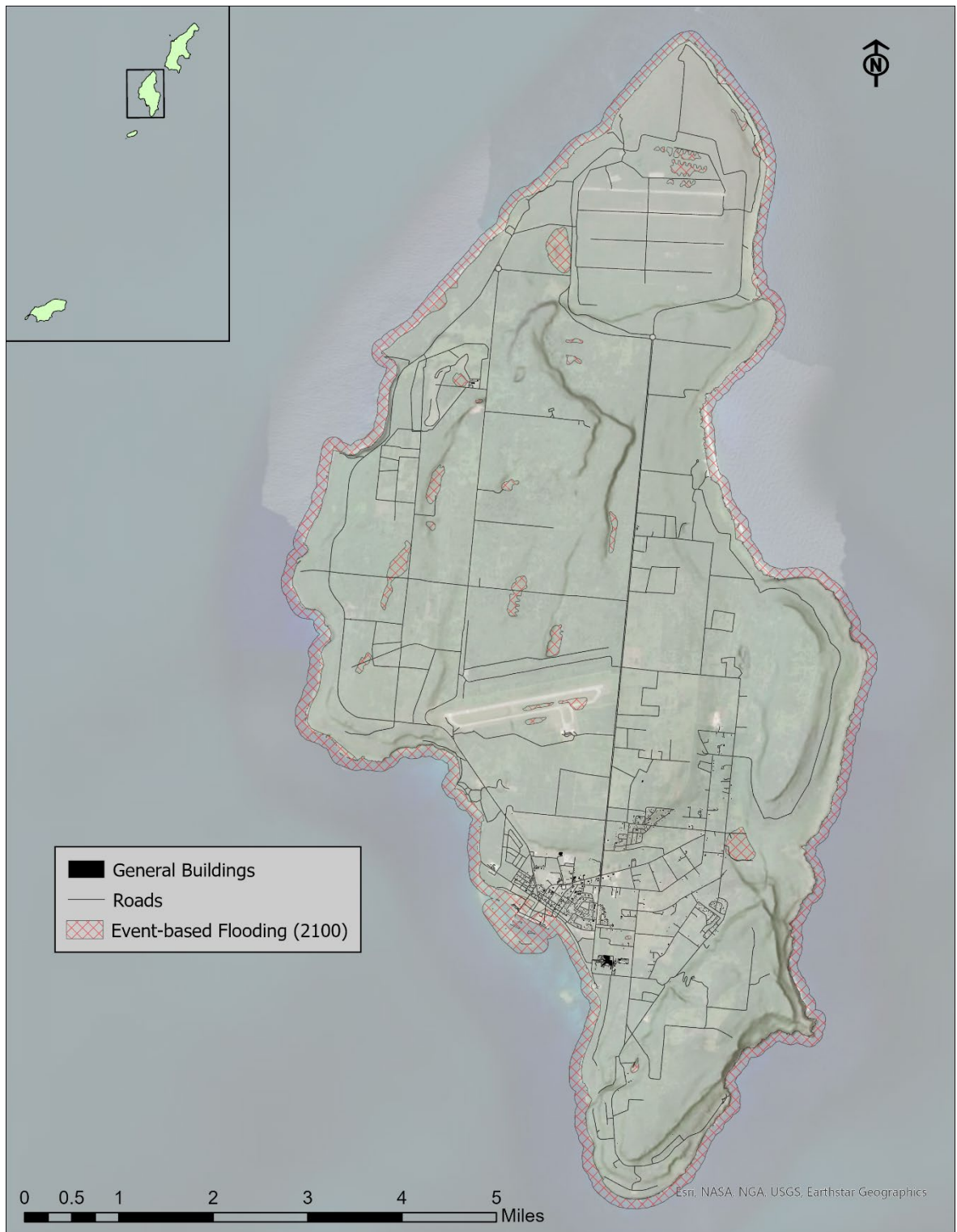
Figure B.5-26. General building stock exposed on Tinian to the future flood hazard including the 1% annual chance flood, 3 ft of sea level rise, and 10% annual chance storm surge.
