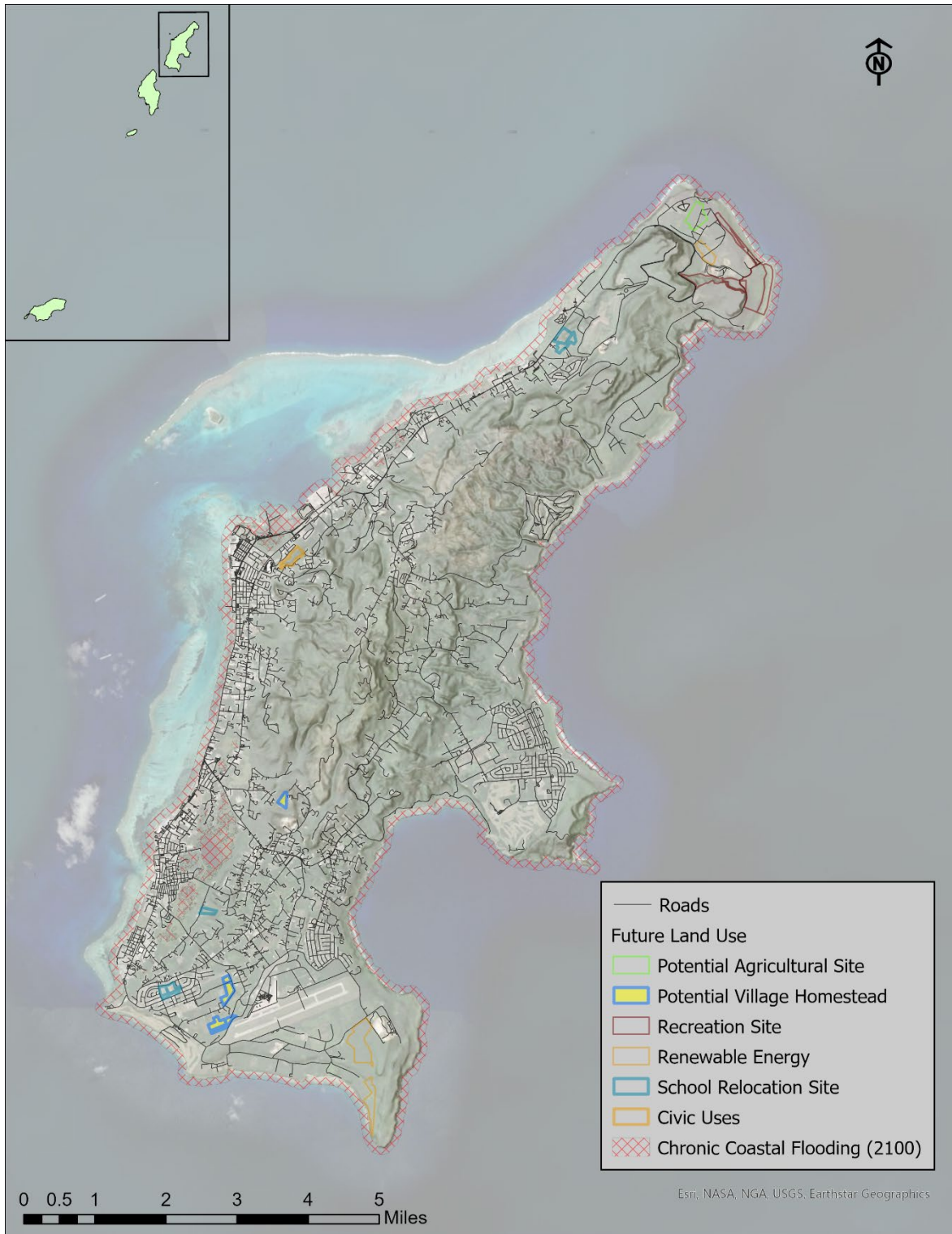
Figure B.5-76. Parcels designated for future development on Saipan exposure to the future chronic coastal flood hazard with 3 ft of sea level rise.
