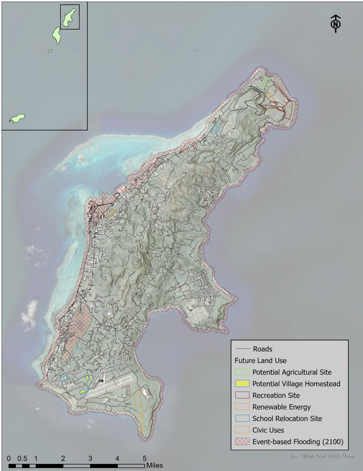
Figure B.5-37. Parcels designated for future development on Saipan exposure to the future flood hazard including the 1% annual chance flood, 3 ft of sea level rise, and 10% annual chance storm surge.
