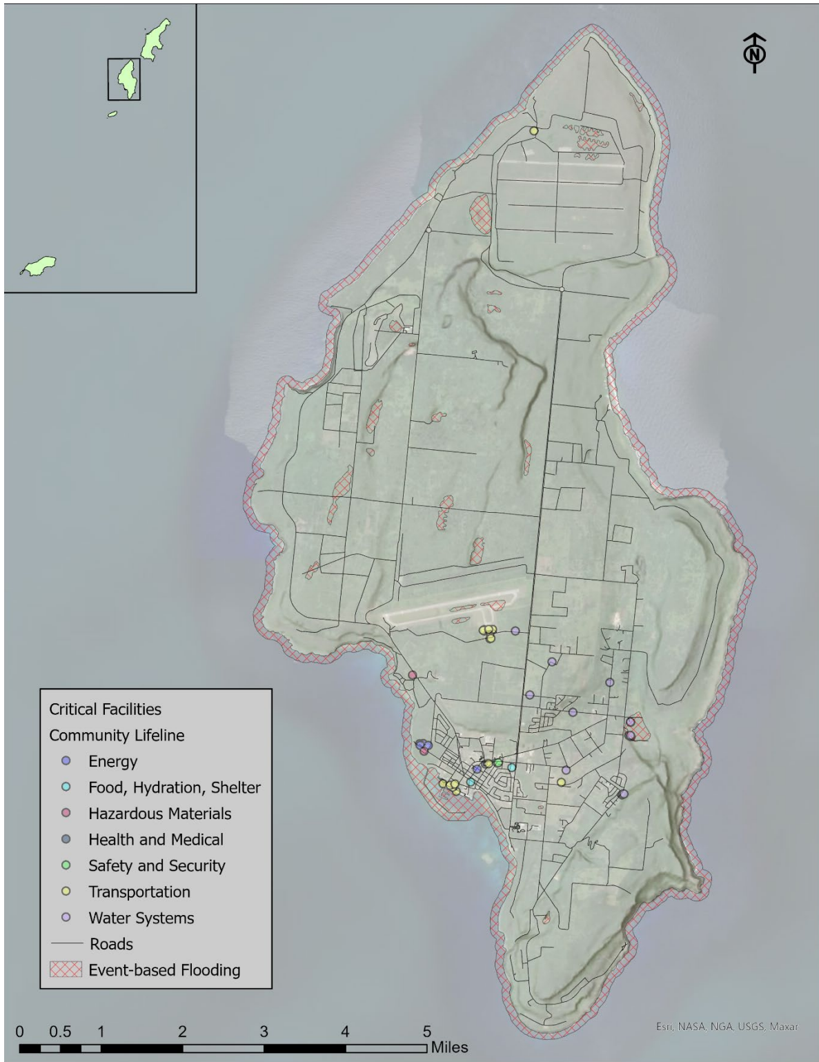
Figure B.5-5. Critical facilities and community lifelines in the Special Flood Hazard Area and exposed to the 1% annual chance event-based flood hazard on Tinian.
