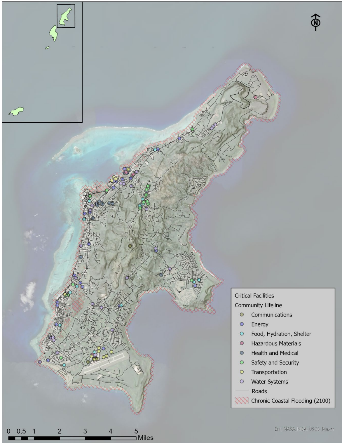
Figure B.5-61. Critical facilities and community lifelines exposed to the future chronic coastal flood hazard with 3 ft of sea level rise on Saipan.
