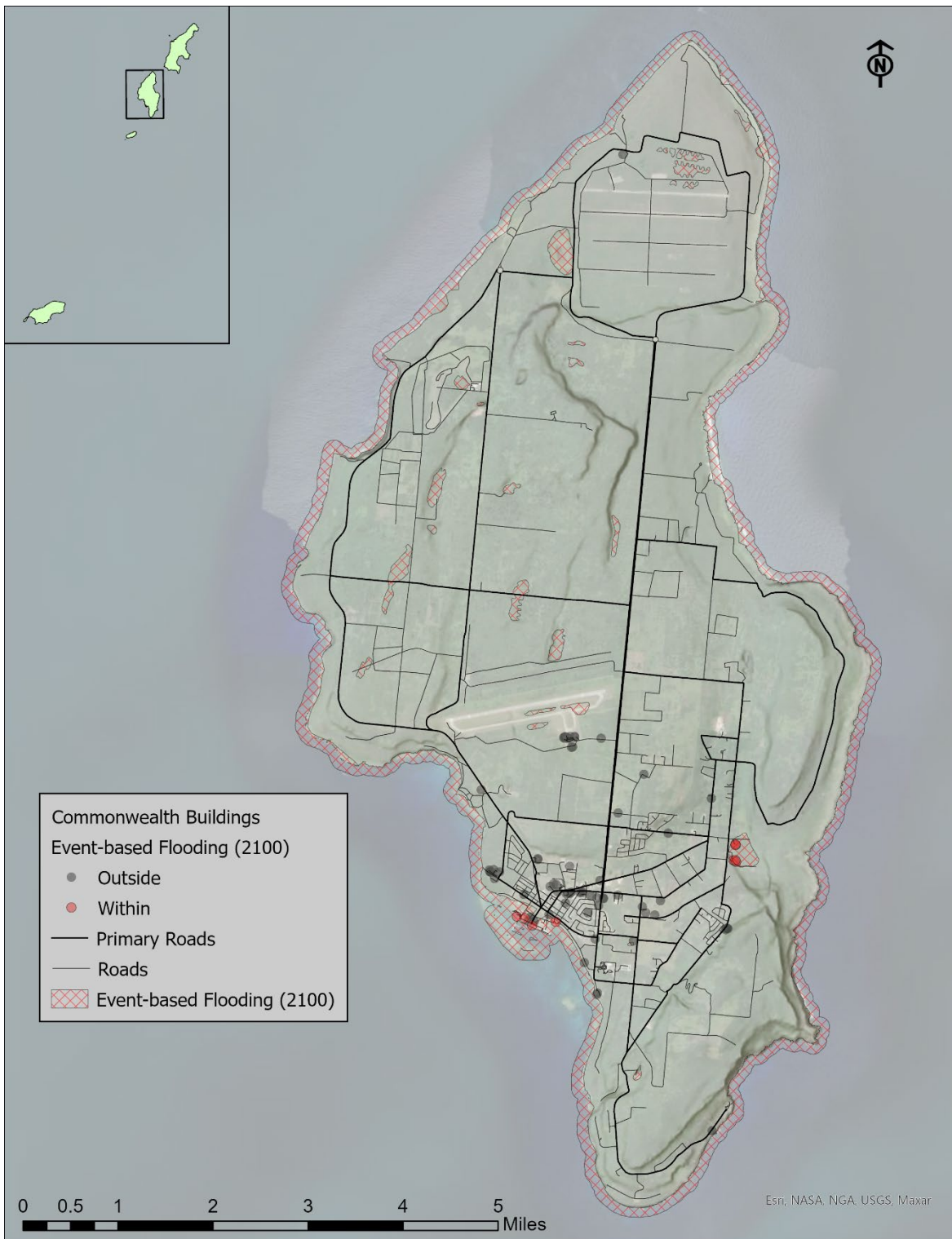
Figure B.5-20. Commonwealth buildings exposed on Tinian to the future flood hazard including the 1% annual chance flood, 3 ft of sea level rise, and 10% annual chance storm surge
