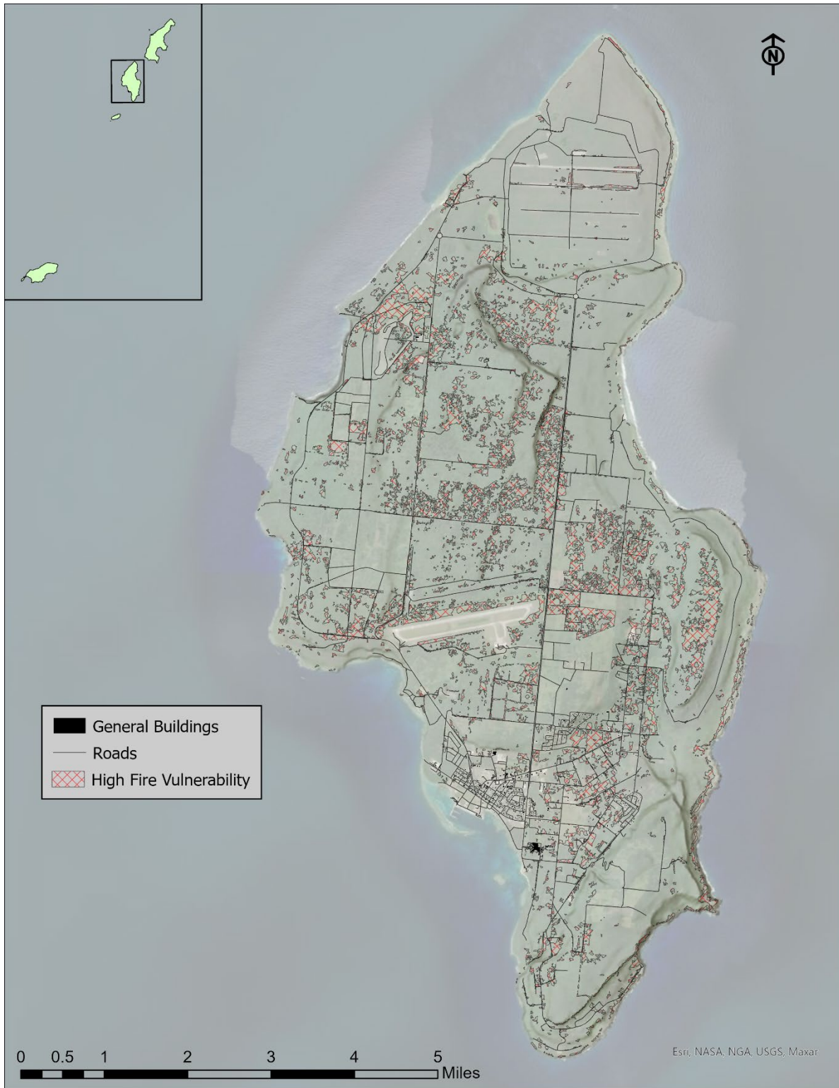
Figure B.8-11. General building stock exposed to the high wildfire probability hazard on Tinian.
