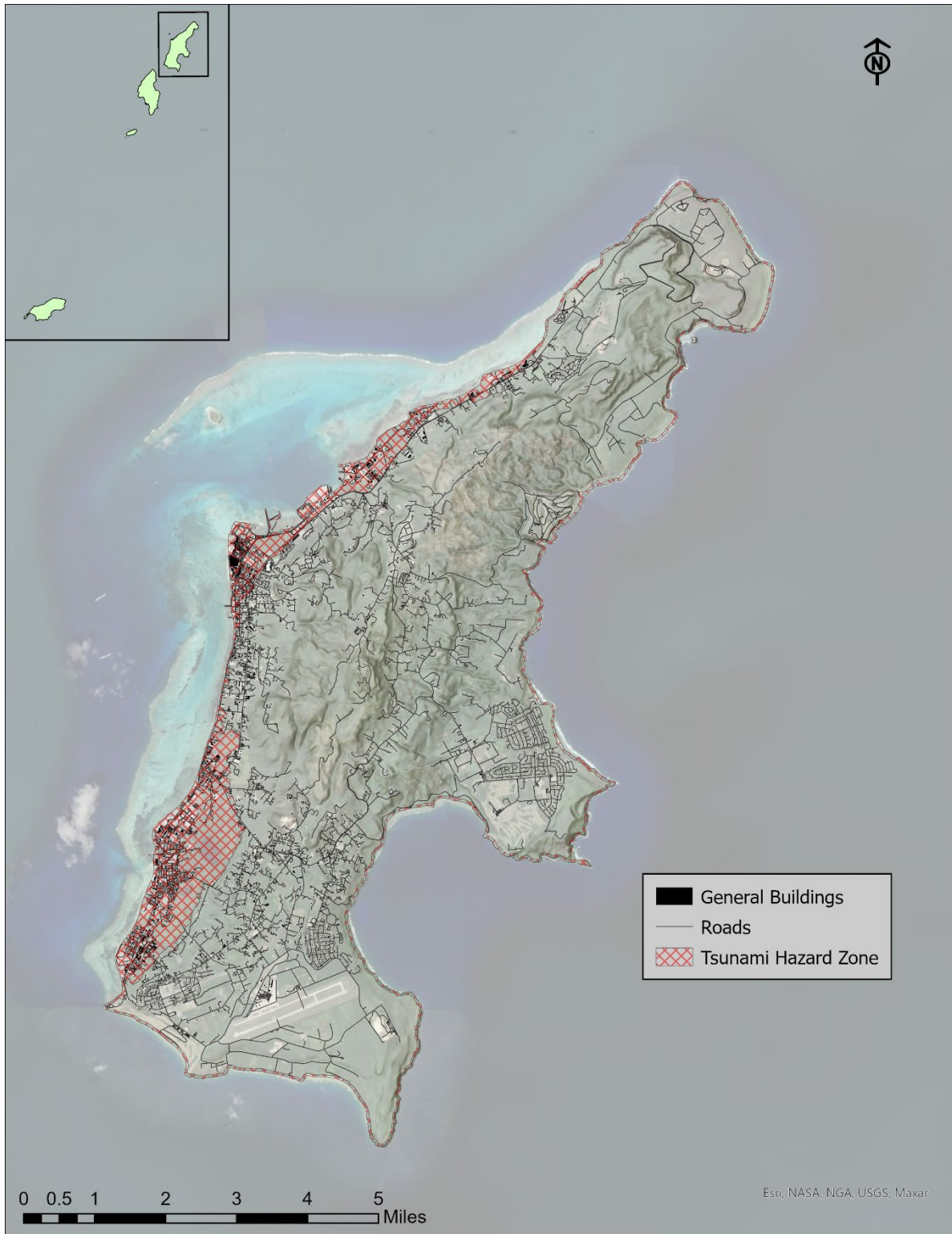
Figure B.3-10. General building stock exposed to the tsunami inundation hazard on Saipan.
