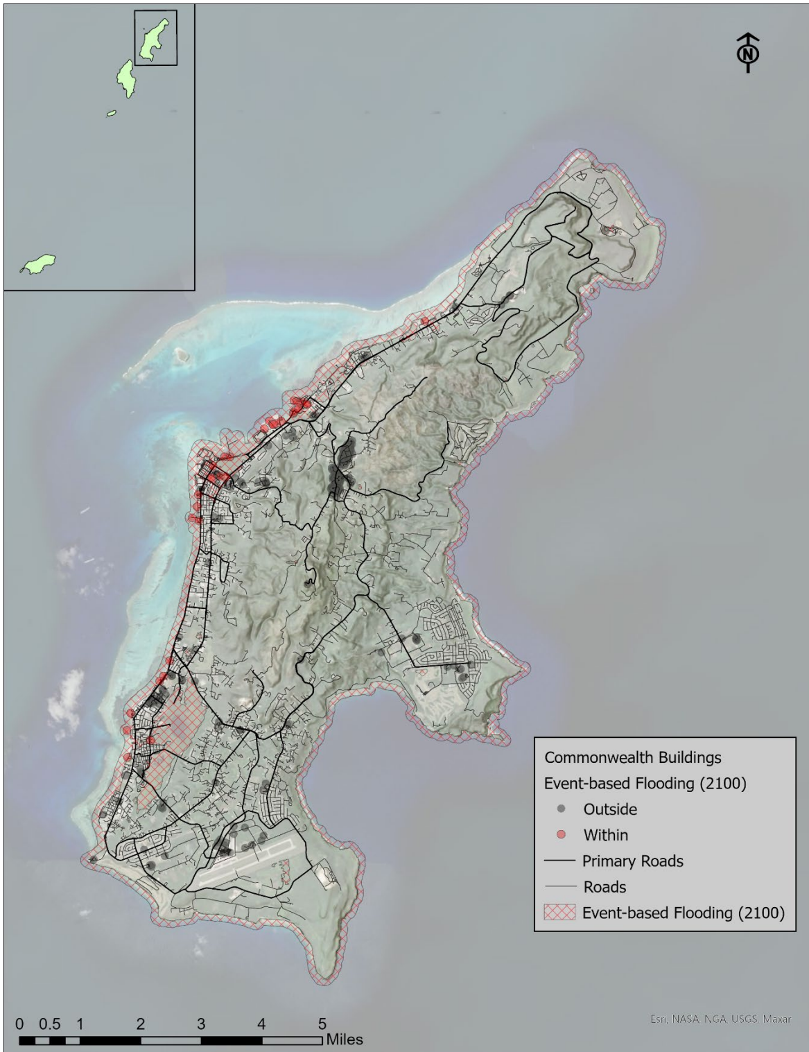
Figure B.5-19. Commonwealth buildings exposed on Saipan to the future flood hazard including the 1% annual chance flood, 3 ft of sea level rise, and 10% annual chance storm surge.
