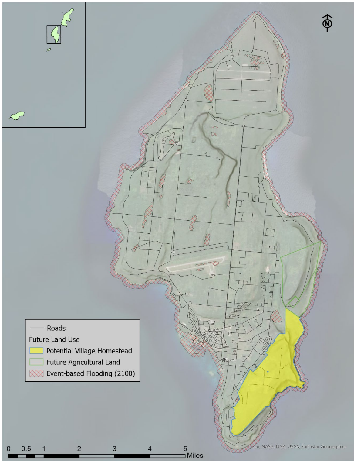
Figure B.5-38. Parcels designated for future development on Tinian exposure to the future flood hazard including the 1% annual chance flood, 3 ft of sea level rise, and 10% annual chance storm surge..
