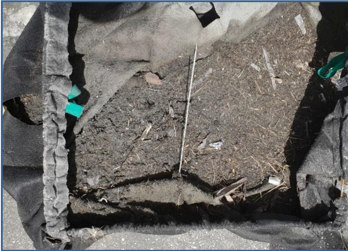
Figure 3. Storm Drain Guard with Captured Sediment
