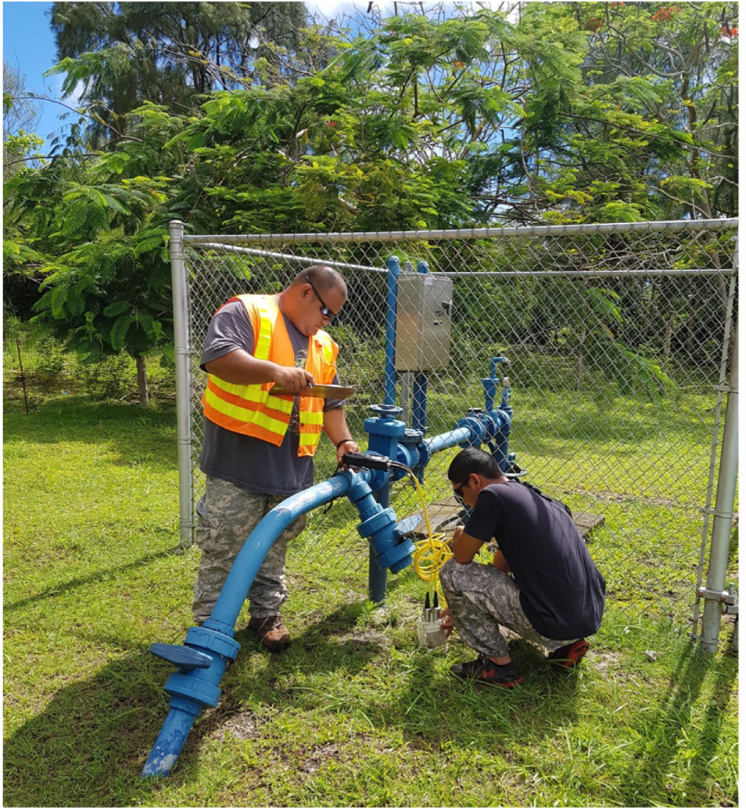
Rota Water Operators Gabriel Dela Cruz and Austin Lizama measure pH and conductivity at a well. During a drought, CUC Rota can use one of their three wells to supplement the primary water source from the Main Cave.
