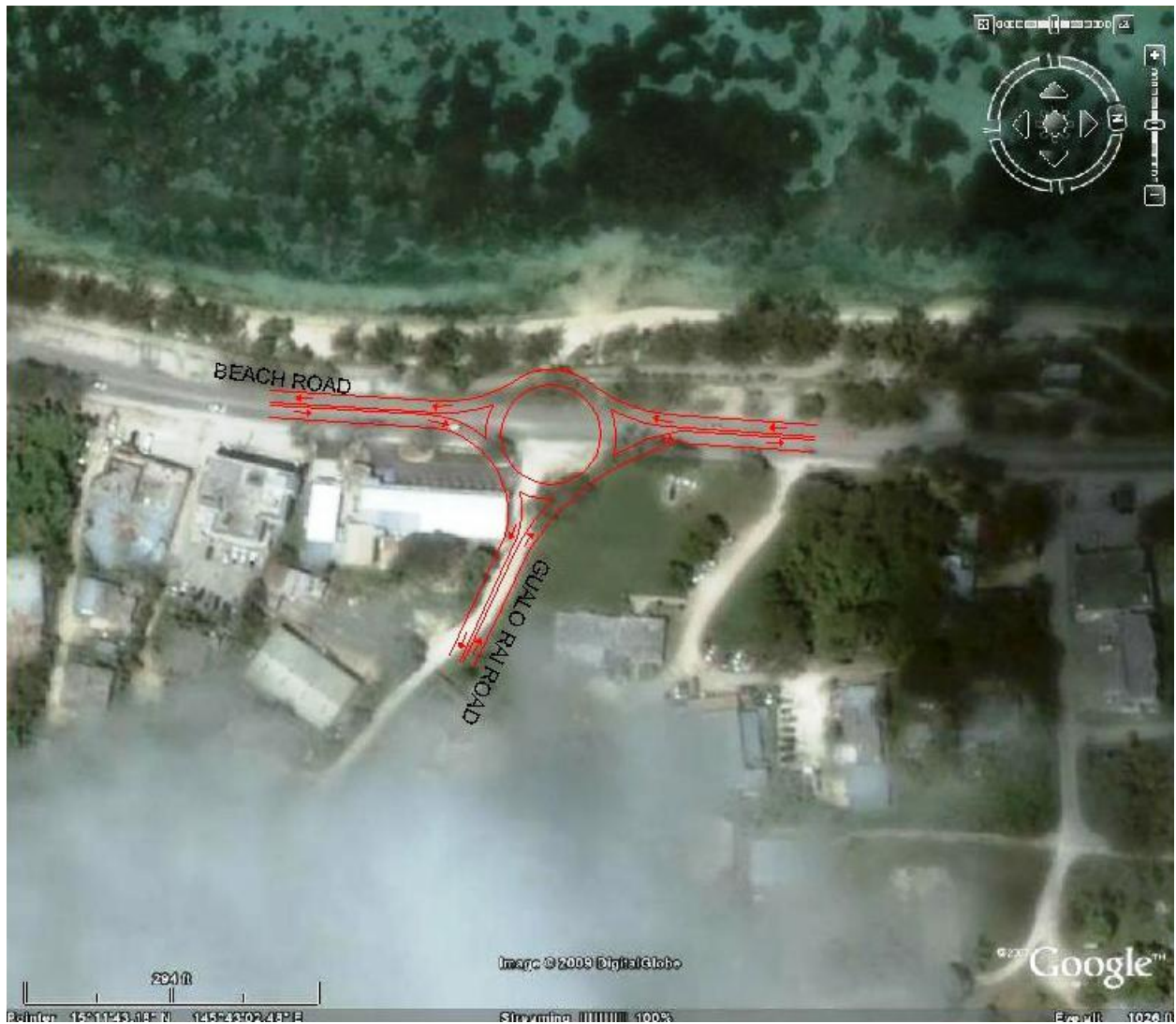
Figure 48: Conceptual Layout of Roundabout at Beach Road and Gualo Rai Road
