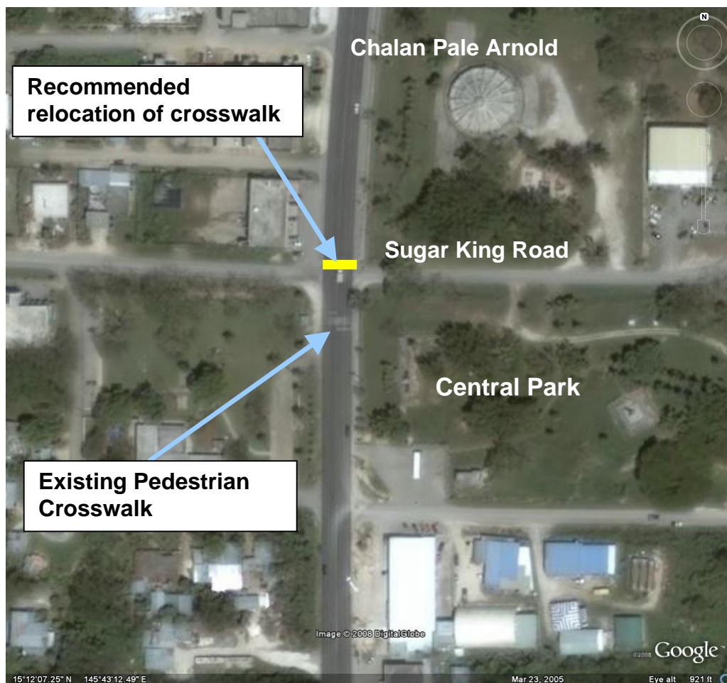
Figure 54: Recommended Crosswalk Relocation on Chalan Pale Arnold
