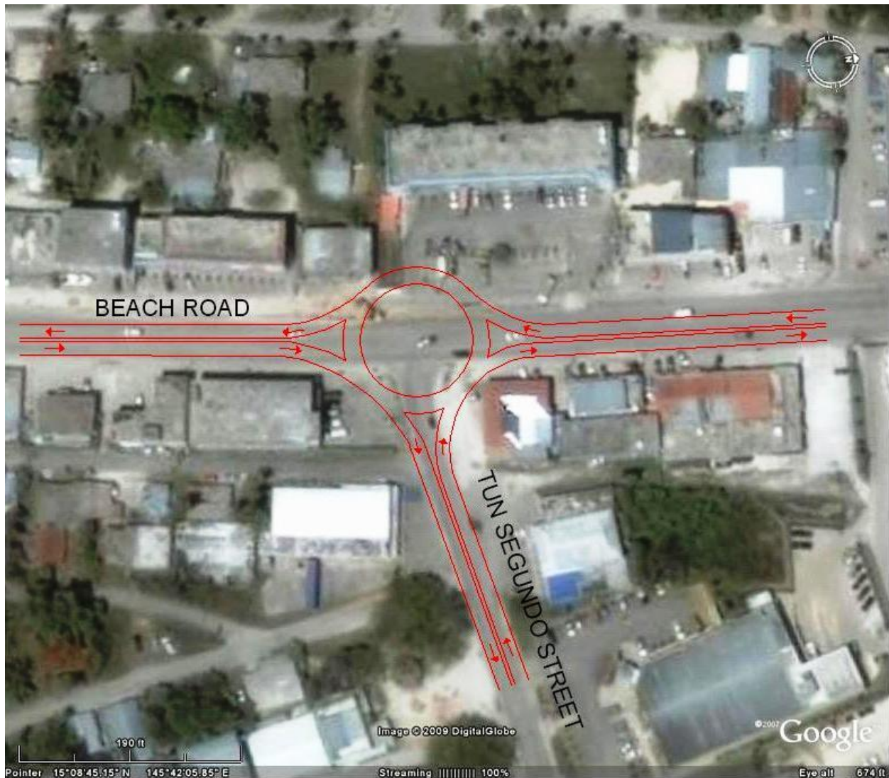
Figure 52: Conceptual Layout of Roundabout at Beach Road and Tun Segundo Street
