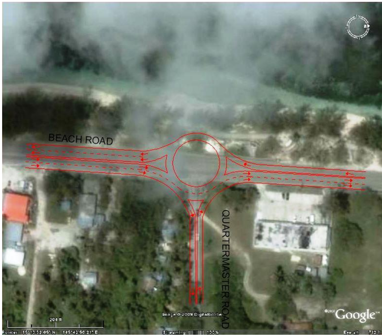
Figure 46: Conceptual Layout of Roundabout at Beach Road and Quartermaster Road
