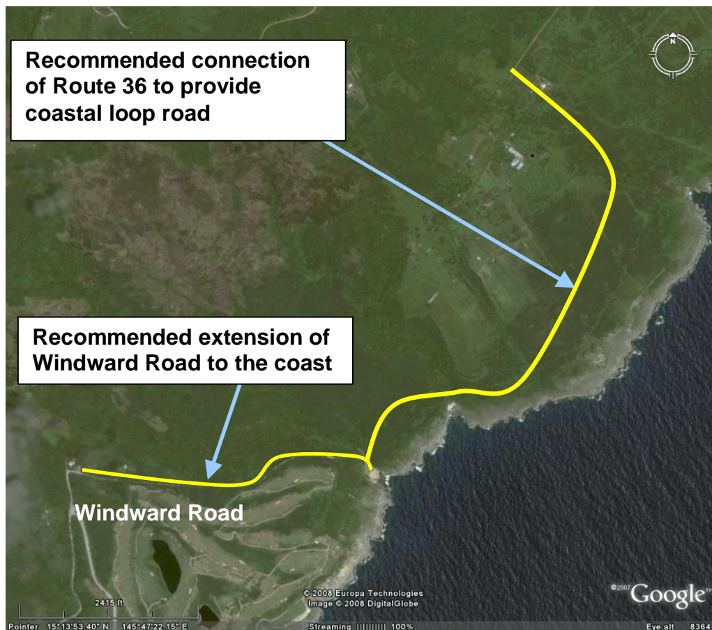
Figure 62: Recommended Improvements on Route 36
