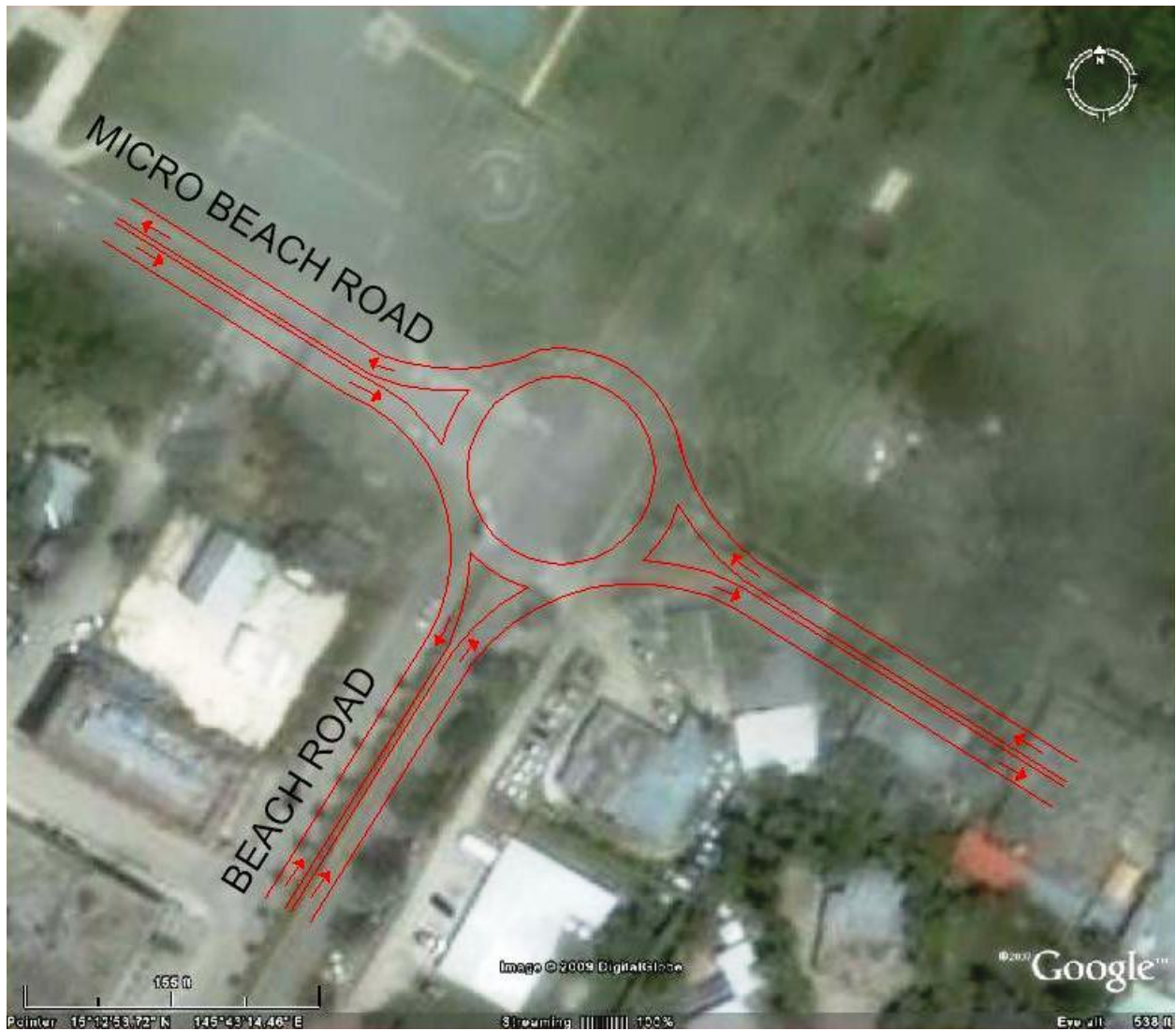
Figure 50: Conceptual Layout of Roundabout at Beach Road and Micro Beach Road
