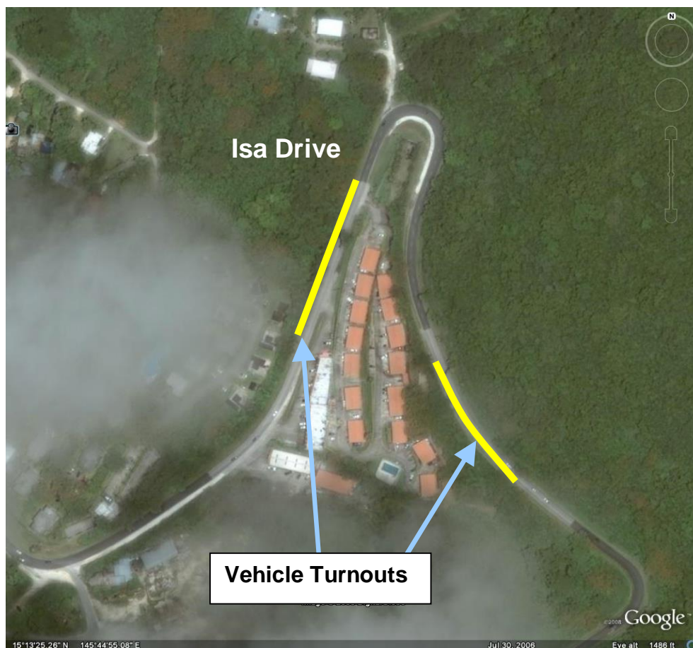
Figure 53: Recommended Vehicle Turnouts on Isa Drive
