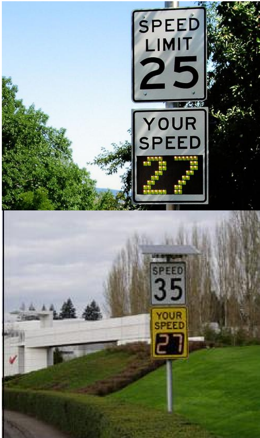
Figure 59: Example of Solar-Powered Radar Speed Sign
