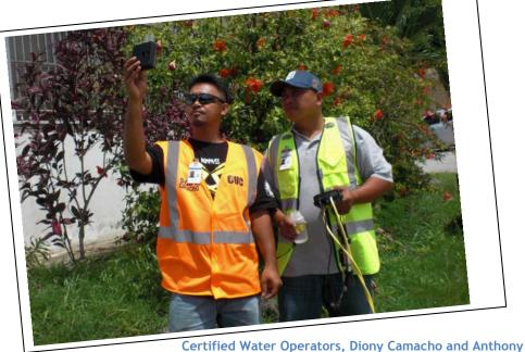
Agulto, measure chlorine and pH in water sample.
