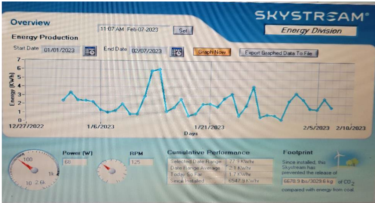
Figure 24. Power production profile for the DPW Skystream wind turbine for January 2023.
