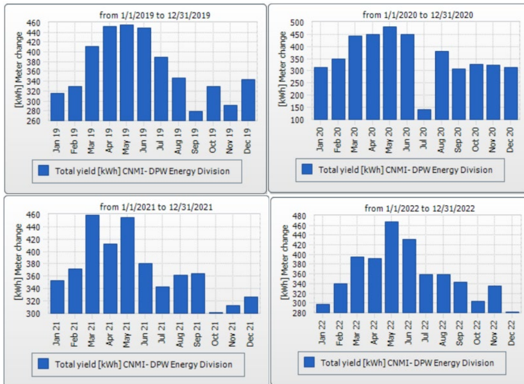
Figure 9. Electricity Production of DPW PV System for 2019–2022 (SunnyPortal 2023)
