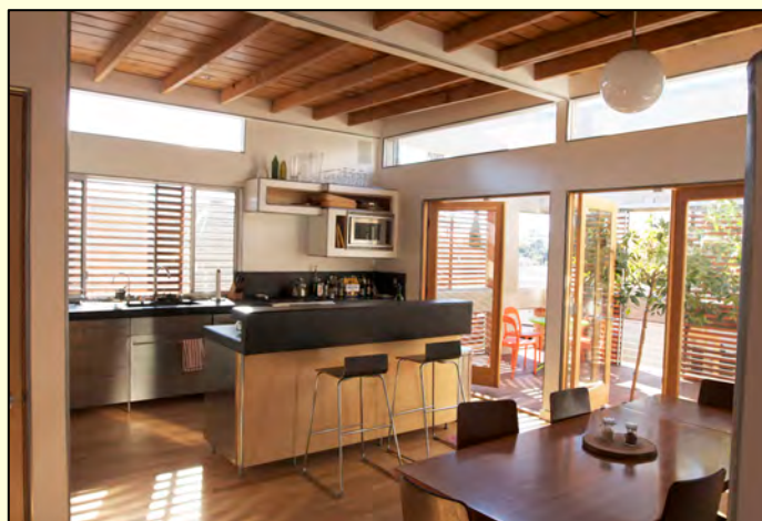
Exhibit 4-18: Sustainably designed kitchen. This kitchen in Eagle Rock, California, uses natural lighting to reduce the need for electricity. Rolling wood screens can be moved to shade the south-facing windows during hot weather, and a tree grows through the outdoor deck to provide additional shade. Sustainable materials were used in the construction, including countertops made with recycled coal fly ash.
