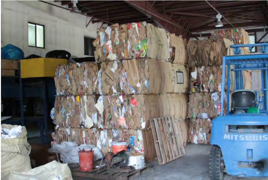
Figure 26. Waste recycling facility equipped with storage capacity for recovered materials
