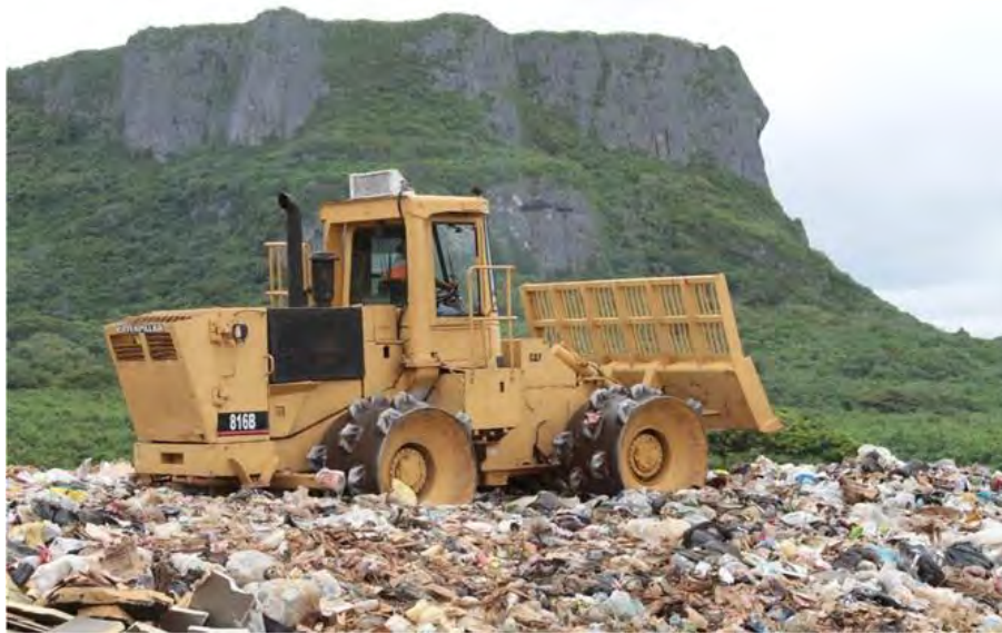
Figure 29. Compactor on working face of landfill at Marpi Landfill in Saipan, CNMI
